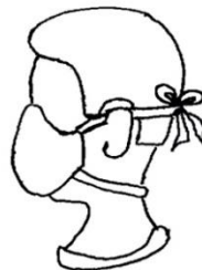
Fastener #2(b) Twill tape/ribbon that ties at the back of the head
