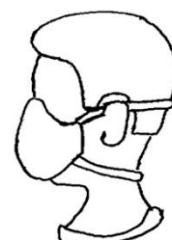
Fastener #3 Elastic that encircles the back of the head & the back of the neck
